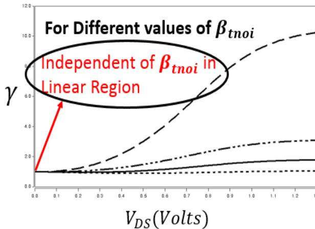
$\gamma$  vs  $V_{DS}$  plots for different values of  $\beta_{tnoi}$ .  $\gamma$  is independent of  $\beta_{tnoi}$  in the linear region and hence follows the  $R_{EFF}$  simulation in Linear region.
