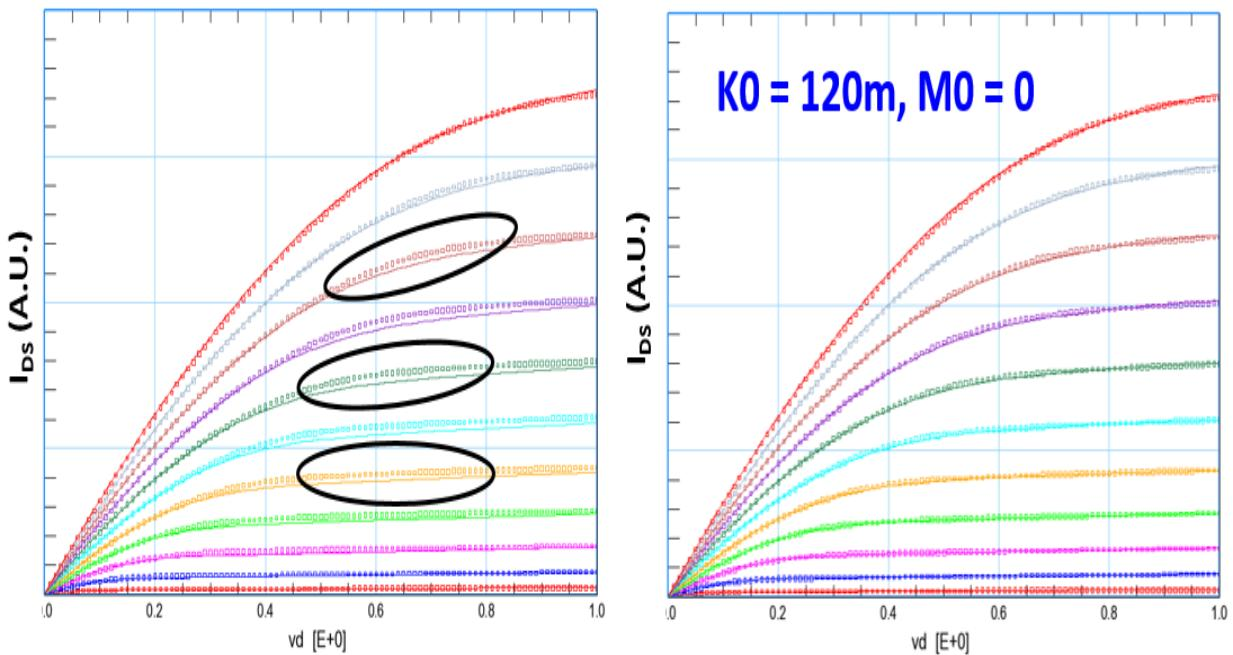
MNUD model improves the  $I_{DS}$ - $V_{DS}$  fitting.
